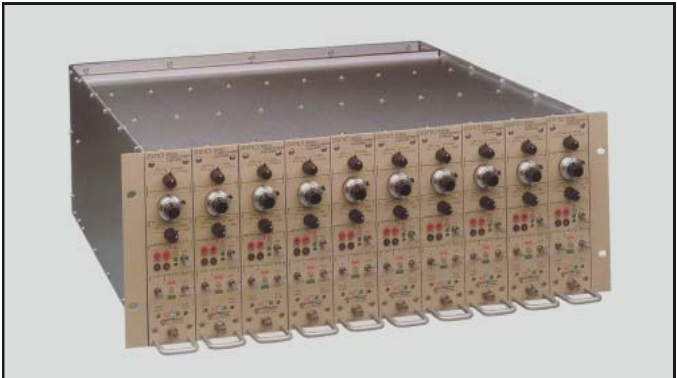
Rack-mounted system allows assembly of signal conditioning amplifier modules for multi-channel testing. Ten-channel system shown in rack. All wiring is built-in to accept adjacent ten-channel systems.
