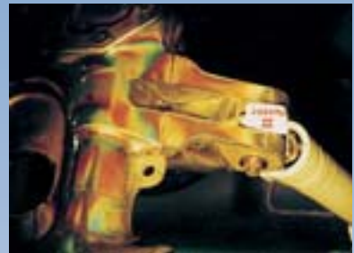
(Right) PhotoStress patterns showing strain distribution over different areas of gear during a load cycle.
