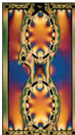
PhotoStress stress patterns of an aircraft fuel door panel under load
