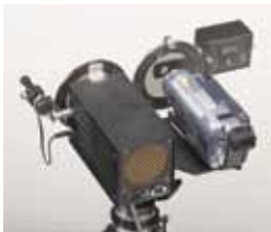
LF/Z-2 Reflection Polariscope—tripod- mounted or handheld
