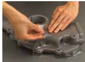
PhotoStress coating applied to a structure of complex shape
