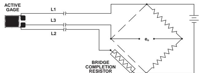
Figure 3. A single self-temperature-compensated strain gage in a three-wire quarter-bridge circuit exemplifies modern strain gage practice for stress analysis measurements.
