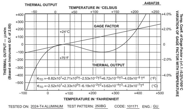
Figure 5. Graph showing typical thermal output and gage factor variation with temperature.
