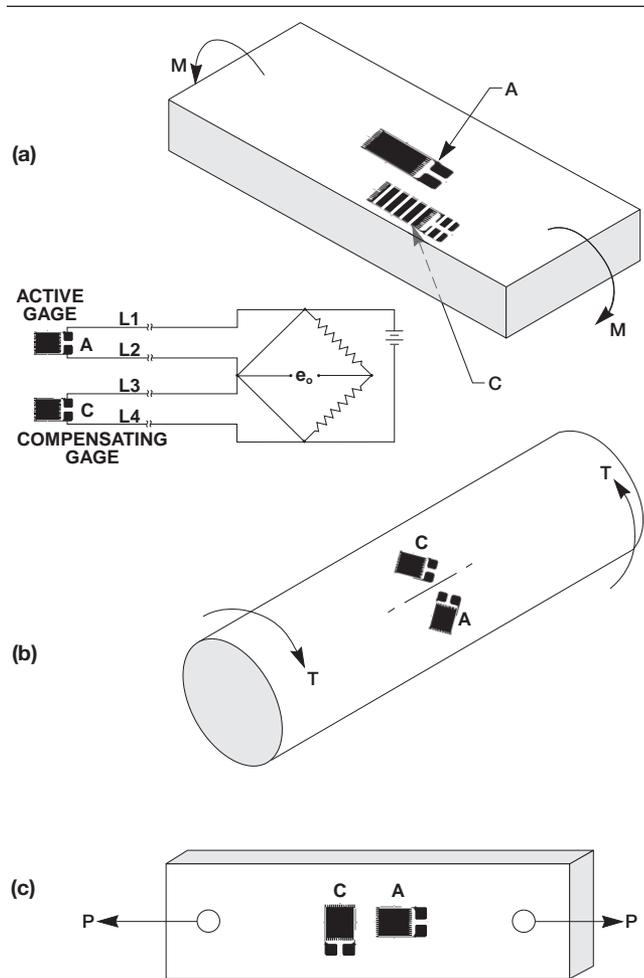
Figure 2. Examples illustrating the use of a second (compensating) strain gage in an adjacent Wheatstone bridge arm to cancel the effect of thermal output.
